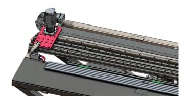
The desired profile positoning will be achieved using the sliding axis on the machine.
