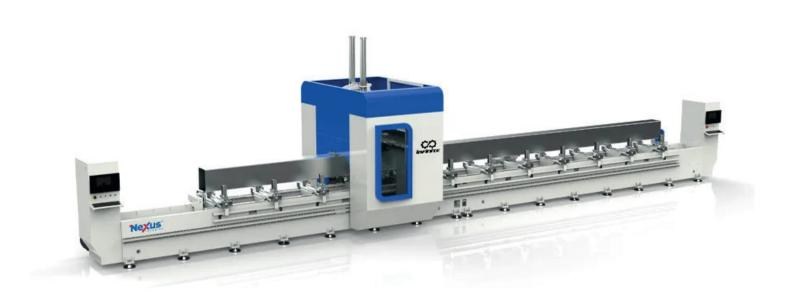
While in the waiting position in the machine park station, the vises are brought into the open positon. The profile to be loaded should be leaned against the fixed front part of the vise. Then, the machine allows the possibility of operation by sending the desired fle from the CAM program.
